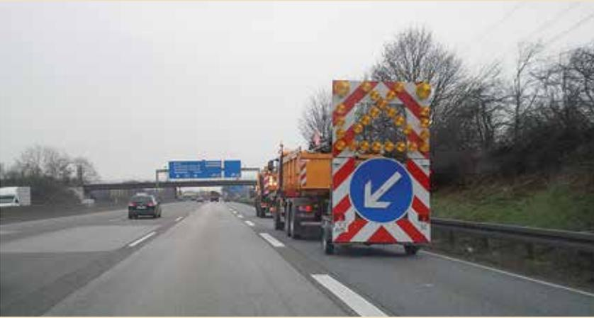
Figure 2: Safety trailer used in Germany
